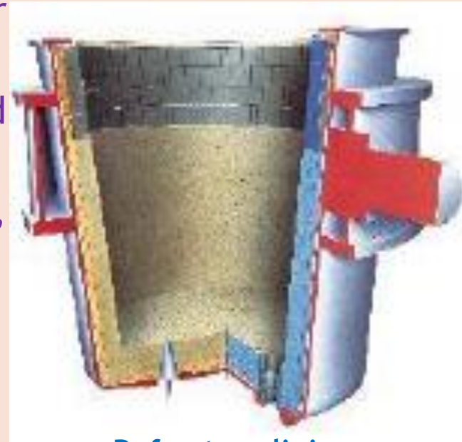
Refractory lining In blast furnace
